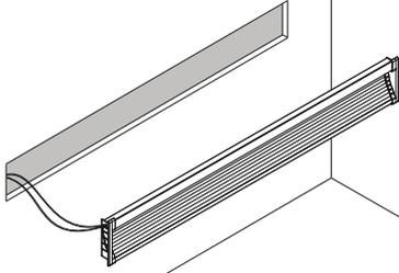
Before fixture is installed, bring low-voltage wires from Alu-Wall through opening in the wall and proceed with wiring to power supply.
