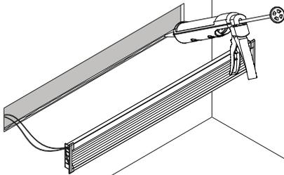
It is recommended that adhesive is applied to the top and bottom surfaces of the drywall opening to secure the extrusion in place.
