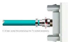
4. At last, screw the wired plug into TV socket accessory.
