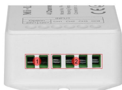
Import port 1. Import power supply cable port 2. Import LED strips connecting port
